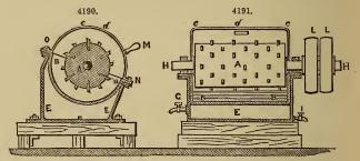
the outer casing B and C which is provided with several projecting diamond-points. The parts of the bundle become heated successively, and, joining together, they at length form a flat lump. This lump, dragged slowly by the powerful friction of the teeth, makes one revolution while the cylinder makes 30 or 40.
